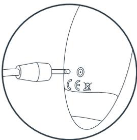
1. The charging port is a small pin hole located on the back. Line up the charging pin with the port.
