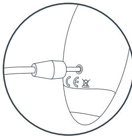
2. Insert the charging pin through the rubber into the port. The rubber will stretch open to accommodate the pin. It's a tight fit!
