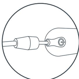
2. Insert the charging pin through the rubber into the port. The rubber will stretch open to accommodate the pin. It's a tight fit!
