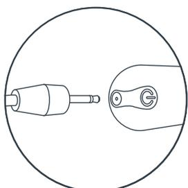
1. The charging port is a small pin hole located below the power button. Line up the charging pin with the port.
